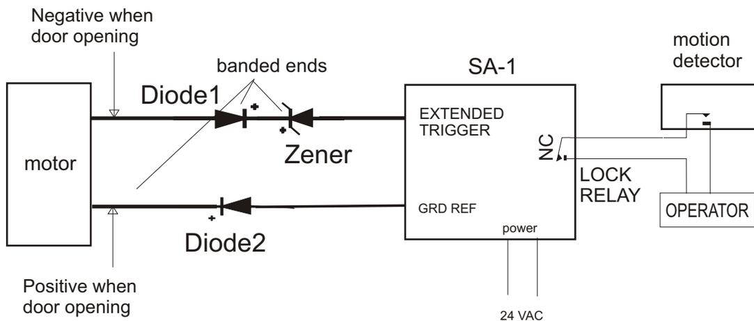
Note the polarity of the DC when the motor is powered for opening.
